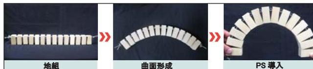
Figure.3 Shape Formation Procedure of PBS
