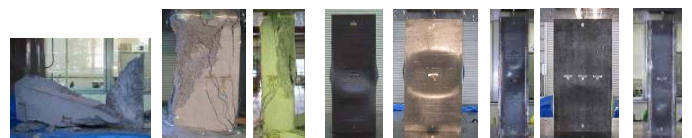
Figure 1. Final failure pattern of plane concrete
