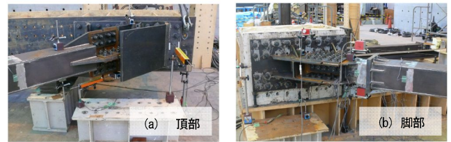
Photo2 Brace to Testing flame Connections
