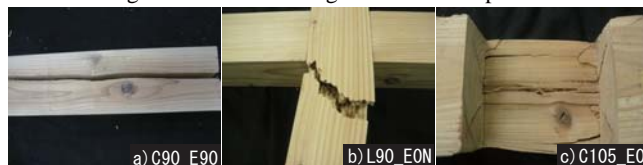
Fig.6 Bending Damage of Test Piece
