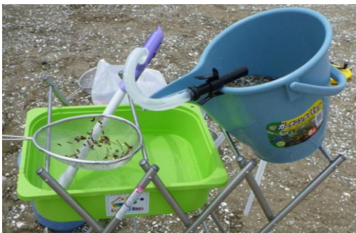
Fig.4 Sorting apparatus using water
