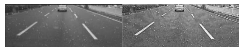
Fig. 1. The processing image of unsharp masking (Left: Original image, Right: Processing image)
