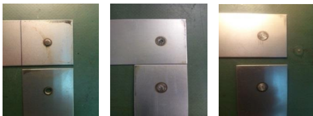
(a) Plug fracture (b) Partly Plug fracture (c) Shear fracture Fig.3 Shapes of fatigue fracture in and around the nugget
