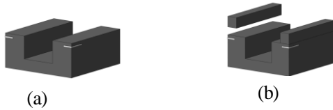
Figure 2. Conceptual diagram of magnetic circuit. (a) Horseshoe shape (b) Stepwise shape
