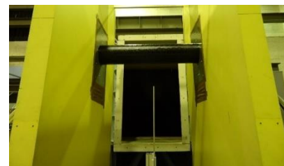
Figure 3. Indented Cable Models and Pitot Tube Anemometer.
