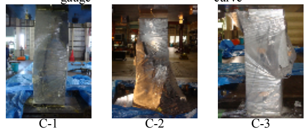
Figure5. Final failure pattern
