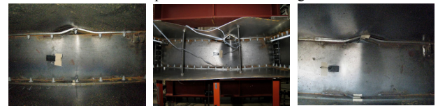
Photo1 Specimen A1~A3 Buckling states
