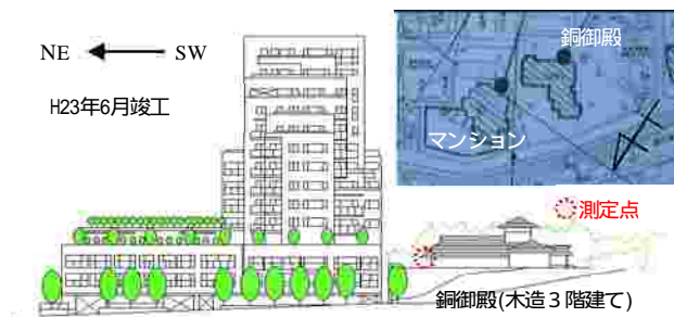
Figure 1. Setting point and those elevation of anemometer
