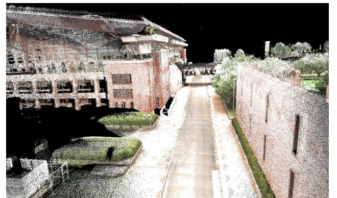
Figure 5. Point Cloud Data at Funabashi Campus
