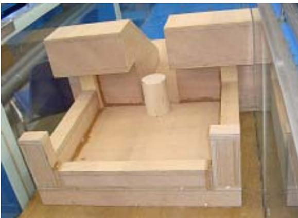
Photo 2 1/6 scale model of pool downstream of weir
