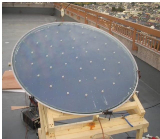
Figure 1. Solar collector of the un-condensing types
