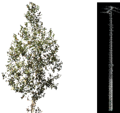
Figure 2. Point Cloud Data on the Tree and the Electric Pole
