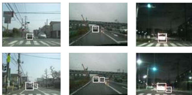
Fig.3 Vehicle detection result by vehicle classifier
