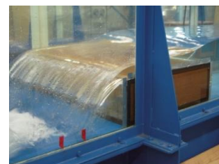
Photo1 Hydraulic Jump immediately below an abrupt drop
