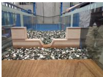
Photo 2 Check dam with compound slit
