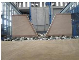
Photo 1 Check dam with trapezoidal slit
