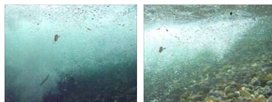
a) Upstream part b) Downstream part Photo 3 Aerated plunging flow below check dam
