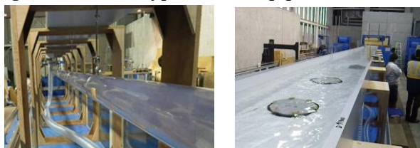
Photo 1 Physical model for drain system network
