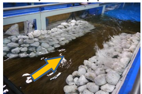
Photo 2 Flow condition in proposed canal
