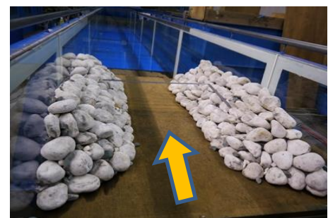
Photo 1 Physical model of proposed canal
