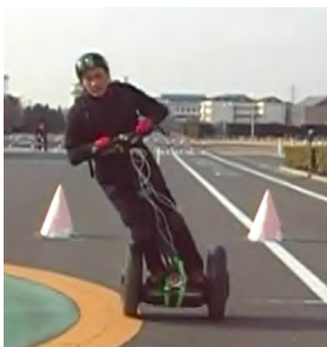
Figure 6. Experiment for driver's feeling at turning safety
