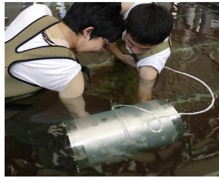
Figure 6. Buoyancy test of one part of AUV body
