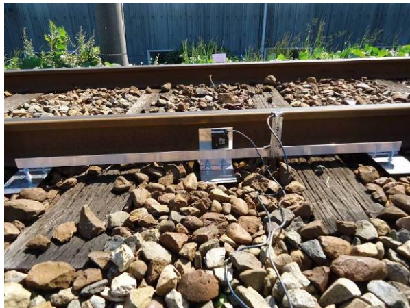
Figure 1. The laser sensor to measure versed sine displacements
