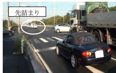
Figure 2. The situation when a vehicle can not enter the intersection because of downstream congestion
