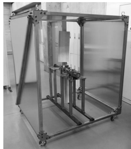
Figure 4 the actual Vibration Control System using Variable Pitch Propeller
