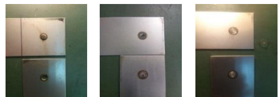
(a) Plug fracture (b) Partly plug fracture (c) Shear fracture
