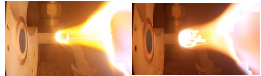
Figure 4. Ablation of Na 2 SO 4 and clay (Left) Ablation of artificial meteor made of Na 2 SO 4 +Clay and Olivine (Right)
