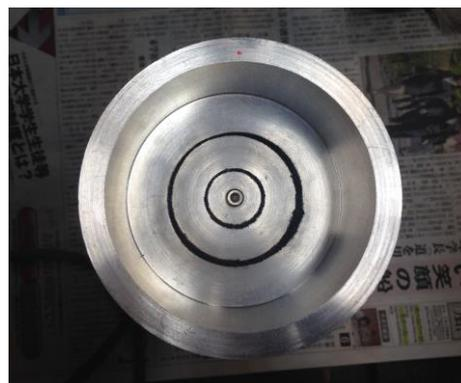
Fig. 3 Sand figure of Chladni on the vibrating plate.
