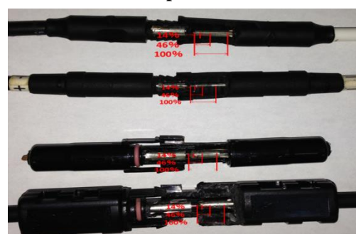
Figure 2. The sectional view of a connector, and the definition of a contact interval (From a top, TypeA, TypeB, TypeC, TypeD)
