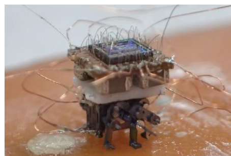
Figure 5. MEMS microrobot with driving circuit.
