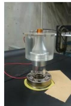
(a) Plasma actuator (b) A nozzle fitted with PA
