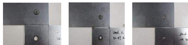
(a) Plug fracture (b) Partly plug fracture (c) Shear fracture
