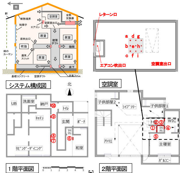
Fig.1 Plan of the house A and measuring points
