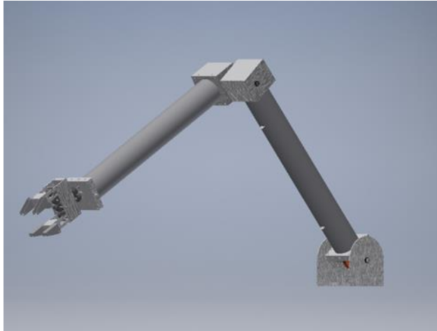
Figure 2 3D-CAD image of the designed robot arm
