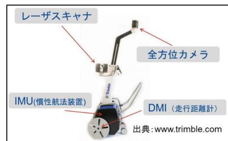
Figure 1. Sensor configuration of TIMMS
