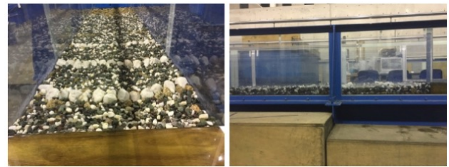
1) bird view from upstream 2) side view Photo 1. The gravel bed with stone-bridges
