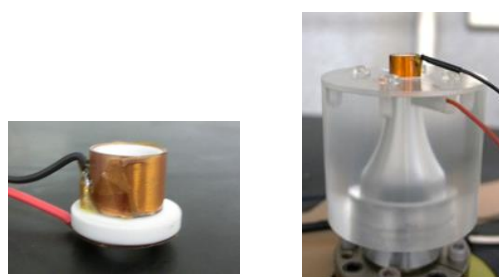
(a) Plasma actuator (b) A nozzle fitted with PA
