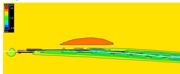
Fig. 4 Contour of |U| around the airfoil, h/c = 3\% , \alpha = 3^\circ
