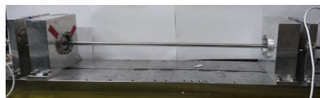
Fig.3 Diagram of designed magnetic bearing device
