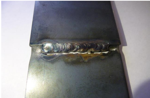
Figure 3. Fractured test specimen
