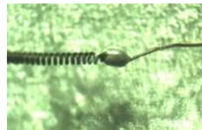
Figure 1. Connection part with conductive paste
