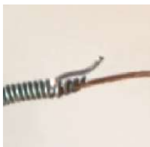
Figure 2. Connection part with spot welding
