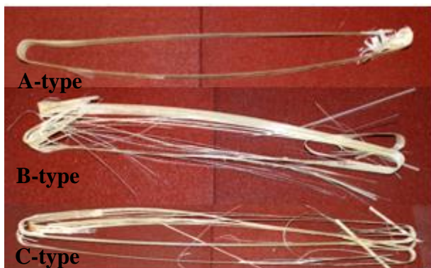
Figure 3. Destructive state of each specimen
