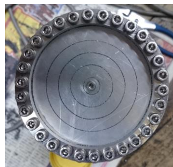
Figure 3. Chladni figure of a vibrating plate plate.
