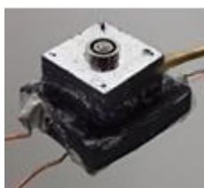
Figure 3. The schematic diagram of the MEMS air turbine micro generator
