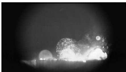
Figure 3. Optical image of bubbles generated piezo nozzle
