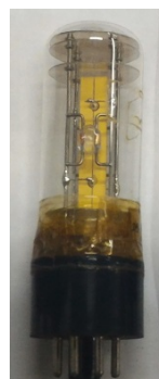
Picture 1 Tube-type resonator (Octal pins)
