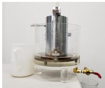
Figure 2. Constant head permeability test
