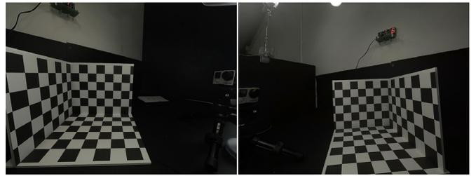
Figure 1. Stereo images of calibration object for a conventional method.
